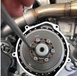
Go ahead and add the weight to the top of the assembly and tighten it back down.
