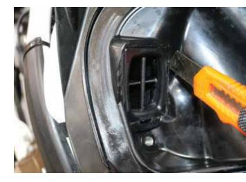
There is nothing holding the reed cage in place other than friction so you can pick it out by digging a screwdriver in the side and prying and also pulling on it and wiggling it out with pliers.cement so it isn't that hard to get out.
