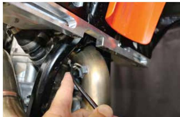
Next you will un-bolt the pipe from the frame. At this point you should be able to just slide the pipe forwards, off of the manifold. You don't have to remove the pipe completely if you don't want to. It's easier to get to the manifold if you do, but I just slide it forward.
