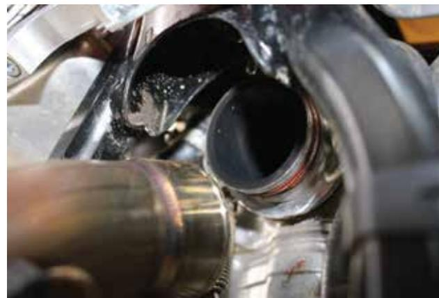
Using grease on the new manifold and the gasket helps a lot as it holds the assembly in place on the cylinder as you are fitting the bolts back into place. You still want to smear a little grease around the O-rings as well, so that the pipe will slide on easier.
