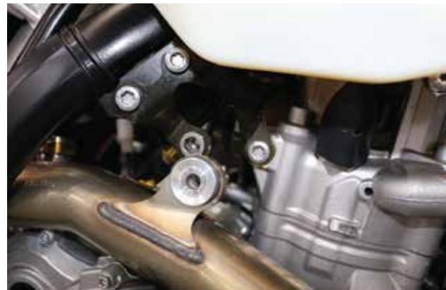
You can get to the two 8mm head bolts that hold the manifold to the cylinder through the front here. **Take them out slowly**, as a few times I've dropped one into the open head pipe. Then you have to take the shock off and the pipe off to get the bolt out. Watch the springs too, if they are still on the flange.
