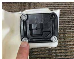
So at this point, you need to get the pump assembly out of the bottom part of the tank. If you have an oversize tank, it will probably just fall out and your good.
